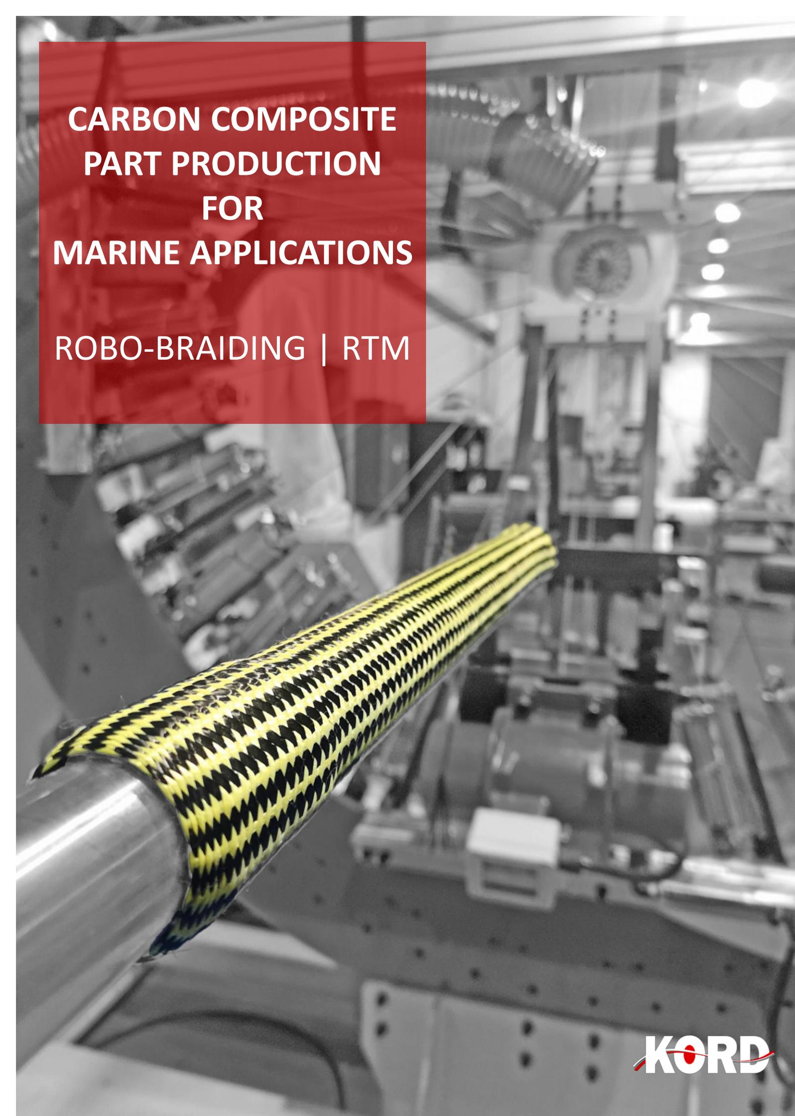
A robotic arm in a factory is shown producing a yellow and black braided carbon composite part. The background is a blurred industrial setting with various machinery and equipment.
