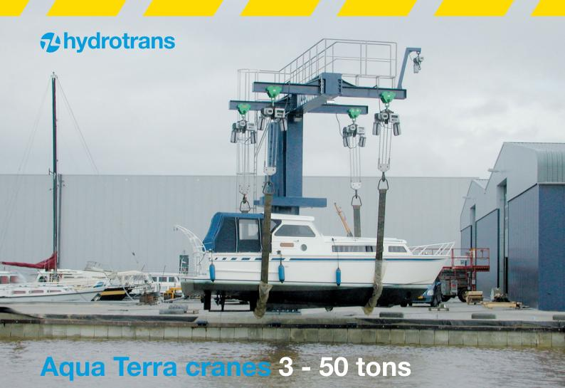
Hydrotrans builds cranes in standard sizes from 3 to 50 ton and can design and build-to-order in larger capacities.
