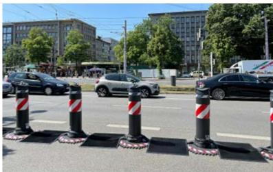
Image 4: As the only bollard-based vehicle barrier with an axisymmetric design, the OktaBlock TR from Hörmann fulfils the requirements of DIN SPEC 91414-1. To obtain DIN SPEC certification, the mobile bollards are connected to
