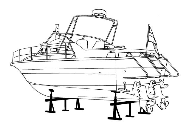
An all-steel bar stand suitable for almost all kinds of motorboats. A variety of models are available to carry loads of 500–10.000 kg each.
