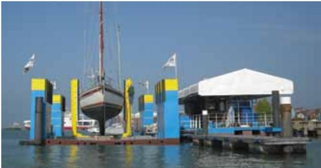
Following the success of its revolutionary Sealift2/RD rolling deck design Sealift2 International Limited is proud to present its new Sealift2/SD shallow draught floating dry dock.
