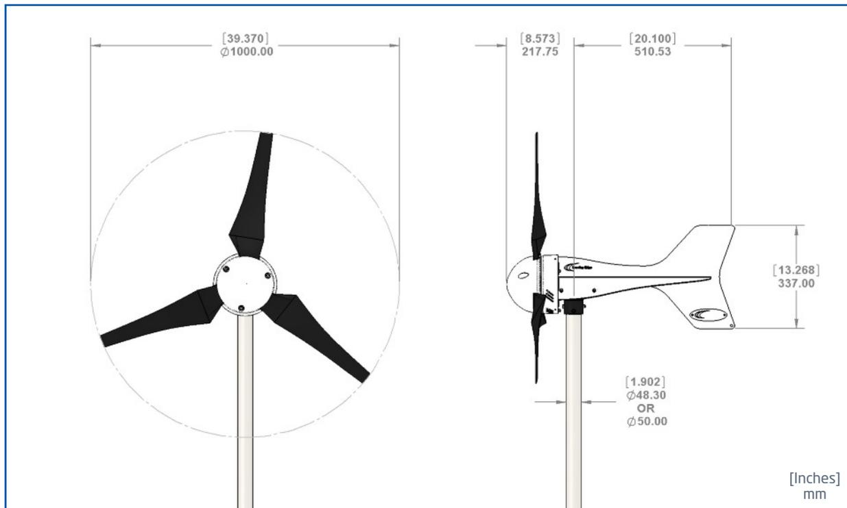
The LE-300 is precision engineered in the UK with only two moving parts so little maintenance is required during the turbine's long operating life. Where wind speeds can regularly reach over 27m/s (60mph), the LE-300 Extreme is the wind turbine of choice.
