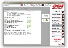
Complete engine tests to review data such as Active Faults, Run Time, and Freeze Frames on the History Tab.
