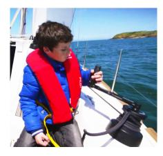
The first two gears are the same speed as a conventional 2 speed winch so you still sheet in by hand before locking it onto the self tailer. The real benefit is how you then continue to wind-in a heavily loaded sheet with so little effort- almost with your fingertips! On conventional winches this would require two hands,
