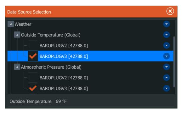
Temperature is included in the information that it sent by the BaroPlug. For best results, place the BaroPlug in a well-ventilated and shaded location.
