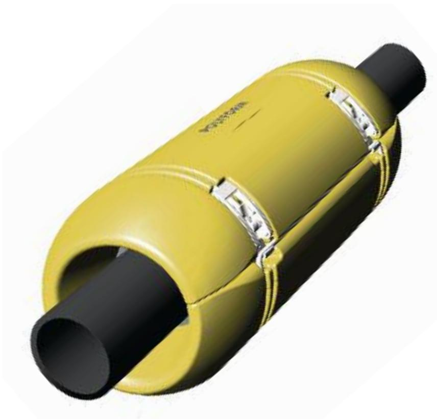
The **POLYFORM® Sub FlowSafe** is made from a rotomolded PE outer shell and filled with polyurethane (PUR) foam, guaranteeing a compressive strength of 500 mH<sub>2</sub>O.
