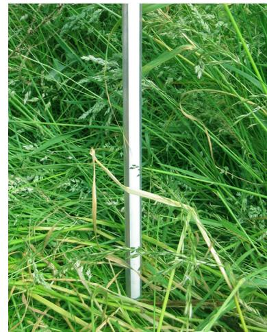
*After 6 months it can be seen that the sensor probe was clean and free from scum/debris build-up.*
