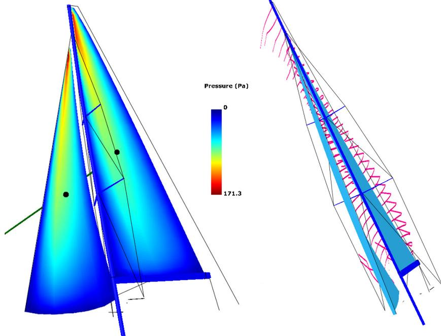
The aerodynamic analysis tools are combined with automated geometry manipulation to enable the SMAR Azure team to analyse a large number of possible sail shapes. In this mode we vary camber, twist, draft as well as sheeting angles. From these results we determine the design that results in the highest drive force, while keeping the heeling moment within the available righting moment
