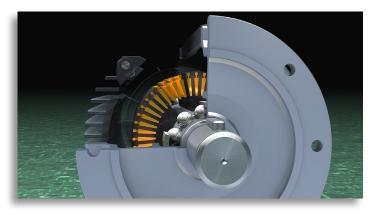
If an electric motor starts to have a problem with a shaft bearing, it is only vibration monitoring that is going to provide you with the necessary indication of a problem. However, if a bearing is starting to fail in a gearbox, it will deposit debris in the oil before it produces a measurable increase in vibration levels.
