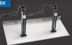
The Lectrotab stainless steel trim tab design provides unmatched strength and reliability. All stainless steel tabs are fabricated with a continuous rolled and pinned hinge, eliminating the need for welding.
