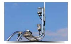
VHF antenna with duplex antenna splitter
