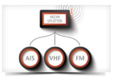
Share a single antenna for VHF radio, AIS and FM/DAB radio
