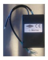
Add-On hardware module with user software for retrofitting existing electricity pedestals to become Internet Of Things.
