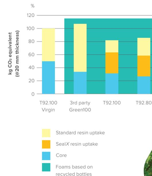
Due to its unparalleled resin uptake, the virgin-PET based **AIREX® T92** version already outperformed the 3<sup>rd</sup> party's PET core materials based on recycled raw material. These sustainable credentials of **T92** are now confirmed and expanded with the renewed, green **AIREX® T92** containing recycled post-consumer bottles.
