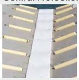
Equipped with stainless steel screws, it is fixed on the central ball joints. Very slippery, it facilitates the ascent and descent of the boat while preventing pins unlocking.
