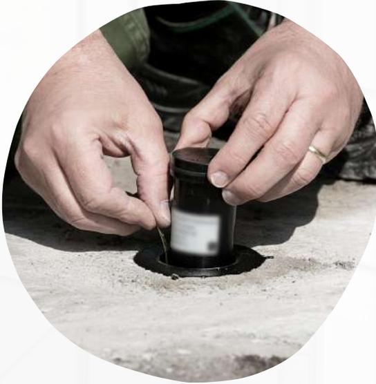
We make urban traffic data easily accessible by using small, easily replaceable, magnetic detection-based traffic monitoring sensors flush-mounted in the road surface.
