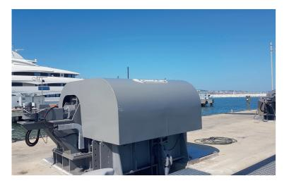
The lifting system is operated by electrically-powered winches controlled in closed loop by inverters. The winches are conceived and manufactured for installation in marine environments.
