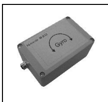
Navio 820 A gyro sensor measures the angle turn per time unit of the ship. By adjusting the rudder against the angle turn, we can minimise the turn. This means that the ship can be steered dead straight down a river without any intervention.
