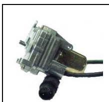
Navio 920 For the control of the fuel motor we use a rotating servo motor. This actuator can be supplied for both a 12 and 24 Volt system. The Navio 920 can be fitted to almost any combustion engine. The full stroke can be travelled within ¼ second. This means that you feel the acceleration immediately, even when accelerating electronically. The Navio 920 can also be used to drive lightweight rudder installations.
