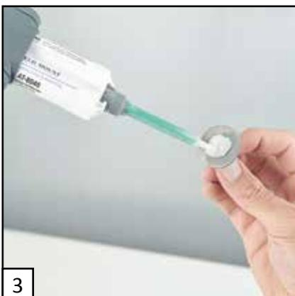
Squeeze the handle to dispense a small amount of adhesive onto the bottom of the part.
