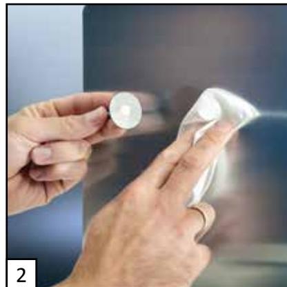
Clean fastener and substrate with scotchbrite and solvent
