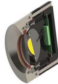
**\*DESCRIPTION** - The QTS-75 range is a submersible through hull marine light with a universal 30 degree ball adjustment. There are two types of insert which have been machined so they can be welded flush to the hull plating at the appropriate locations. Final adjustment of the beam angle to the horizontal is carried out from inside the hull. See instructional picture below.
