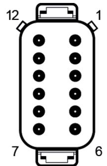
**Please note:** Pins 1 and 5, 2 and 6 must be connected for operation.
