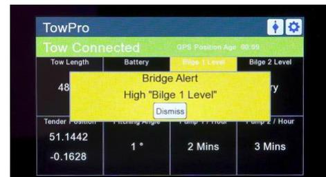
Essential data identified in the Advanced Tow Protection collaboration transmitted live from the tender includes information about how long the bilge pumps have run in the past hour, bilge water levels, battery charge, as well as external factors including continuous measurement of surfing and yawing, trim and pitch, list angle and rolling. All of these are considered key safety indicators of emerging problems with the tow. which can be viewed on TowPro's screen display on the superyacht.
