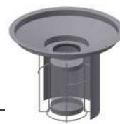
Floating device stops suction when container is full
