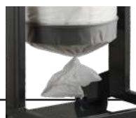
Safe dust collection with Longopac bag
