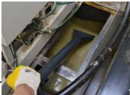
Sludge removal from CNC collection tanks
