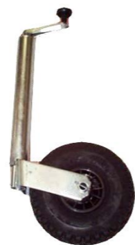
| Inflatable Jockey wheel Ø48 Roller 260 x 85mm Max payload: 120 kg Weight 5 kg T-13082
