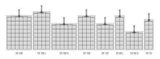
In the SX series the monocrystalline solar cells are electrically connected using ultra-thin copper wires that form a very fine mesh on the cell surface, resulting in thousands of contact connected points. This alternative to the standard bus-bar method allows a higher module power and increases the energy yield. A technology optimally suited to fexible modules, thanks to its intrinsic insensitivity to micro-cracks, that are the most common cause of energy loss in solar modules.
