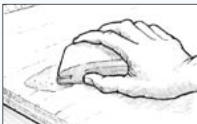
Figure 23 Sand cured fairing compound to desired contour.
