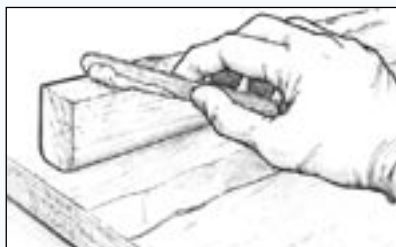
Figure 10 Apply thickened epoxy to one of the bonding surfaces.
