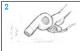
Figure 7 Dry the Surface. Allow wet surfaces to dry thoroughly or use heat or a fan to speed the drying.
