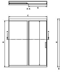
Composed by 2 glass panels, I fixed and the other that slides upon the fixed one. When close, wings keep the surface flat.
