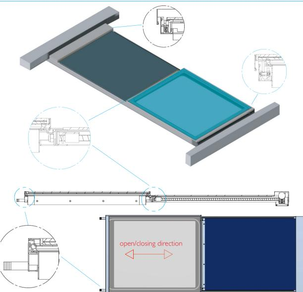
Based on a screwed spindle and nut mechanism, the Sunroof Hatch is characterized by a smart system which press the gasket during the closing operation and made a perfect weathertight and gastight seal.
