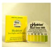
Shows how many parts per million of active antimicrobial you are applying whilst fogging, wiping etc. Shows when rooms are safe for reoccupation after antimicrobial treatments have been used. Very effective when using the Formula 429 antimicrobial family of products. Look for 600 parts per million to ensure good infection standards are met.
