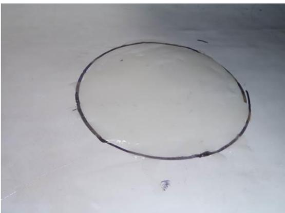
*After preparing the hull area, place the transducer and nut in the proposed position and draw around the outside of the nut to give you a guide.*
