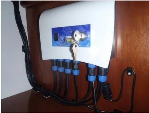
*The unit above was installed in the aft port cabin on the outside of a locker, this gave good access to the main control panel, battery and also the Aft transducers*
