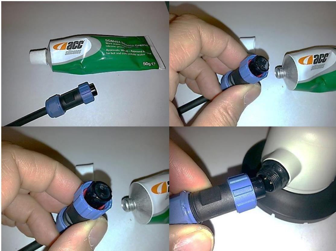
Apply only a small amount of silicon grease (approx. ½ pea or 0.5g) to the plug, ensure the grease is evenly spread over the connection. Then connect plug to socket.
