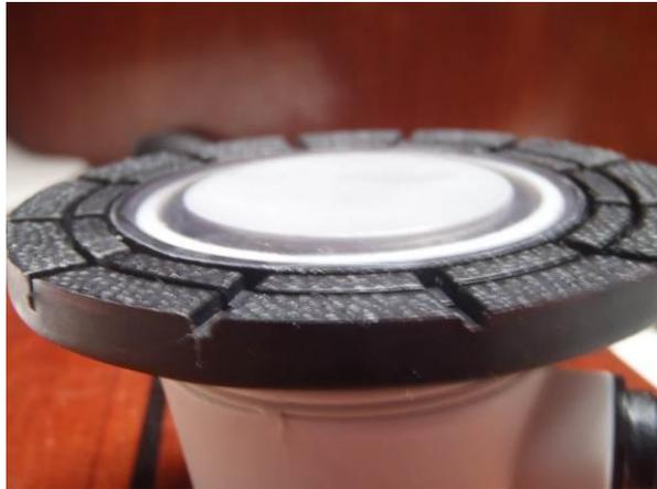
The purpose of the plastic disc is to ensure you have a solid contact to the hull of the boat. Later in this guide you will be applying epoxy resin to the boats hull and this plastic disc will protect the transducer face from the epoxy resin.
