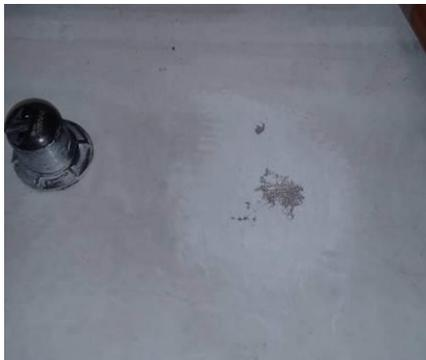
*This area was prepared for the bow transducer using a sander. The more paint you remove the better the adhesion will be.*
