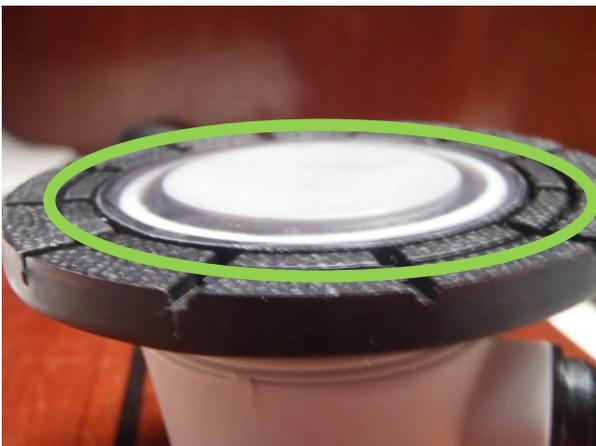
*Apply epoxy to the ring area only (highlighted Green), avoiding contact with the plastic covering (highlighted red below)*
