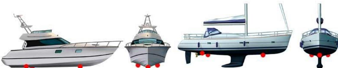
The transducers should be located towards the stern between the propeller and the rudder. One should be placed to port and the other to starboard approximately 30cm from the centre line.
