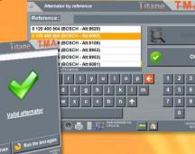
TITANE computer checks all the signals delivered by the tested device. It displays and prints results and performance curves.
