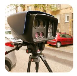
Adaptive Recognition S1 is a mobile no-staff speed and traffic enforcement device with on-board ANPR. It is capable of detecting traffic violations like the abuse of bus lanes or red light crossings and measuring speed from a whopping distance of 1200 meters (4000 feet).
