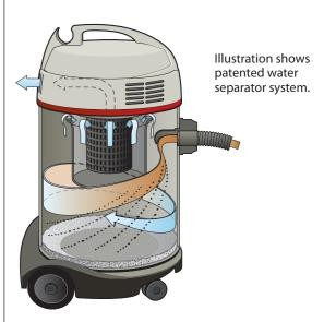
Due to the twist of the intake nozzle, the spray-fog is consequently separated when it reaches the container wall. Additional filters are no longer necessary.
