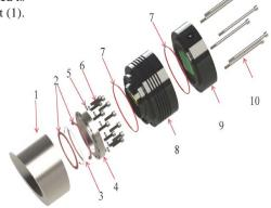
\* LENS FITTING INSTRUCTIONS-Remove the blanking plate and check the insert (1) lens landing surfaces are clean and apply a suitable silicone grease to the gaskets (2). Fit the lens (3), gaskets (2) and lens retaining ring (4). Hand tighten the cap head bolts (6) and spring washers (S.S only 5) making sure the lens retaining ring (4) is square. Torque the bolts to 7 Nm (4.5ft/lbs) in the sequence shown above. Check the ring again and re-torque the screws again to the same setting.
