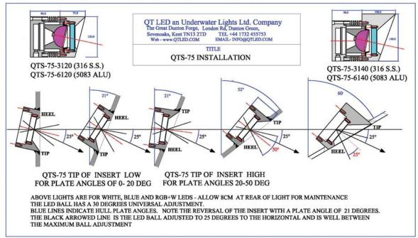
\* LED PROJECTOR FITTING INSTRUCTIONS-The LED heat sink (8) with the 'O'ring (7) fitted is inserted into the insert (1) and loosly held in place by a bolt (10) so the LED ball can be adjusted. The cover (9) with the 'O' ring fitted is inserted to the LED heat sink (8) and bolted up securing all parts to the insert (1).
