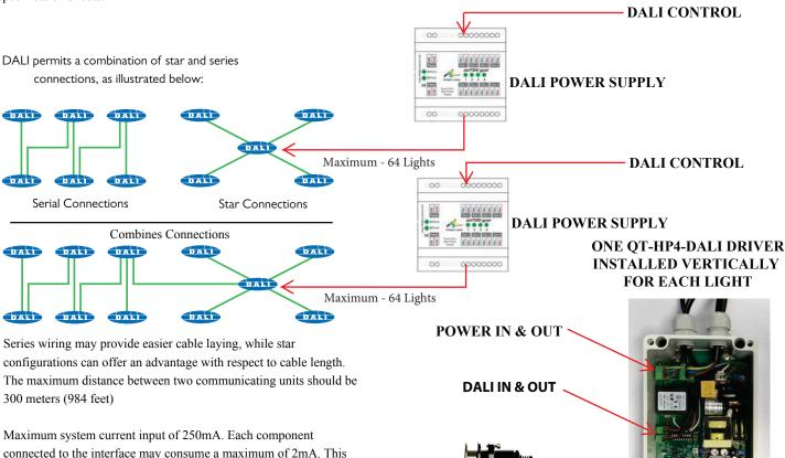
Maximum system current input of 250mA. Each component connected to the interface may consume a maximum of 2mA. This must be taken into consideration when selecting the power supply. Maximum number of 64 units with an individual address.
