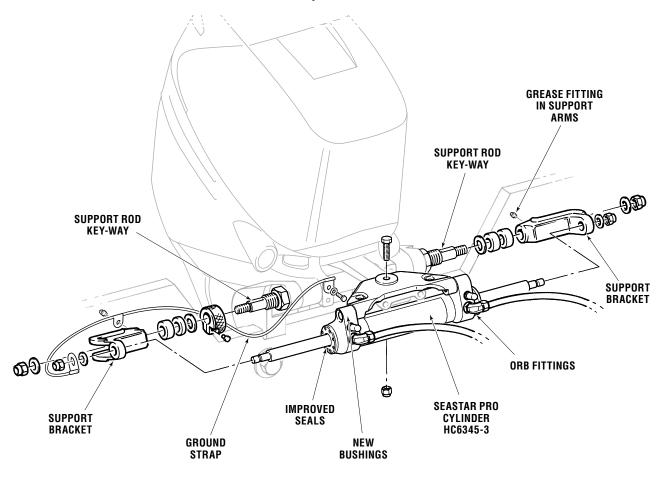
Figure 3-6. Cylinder Part# HC6345-3 shown.
