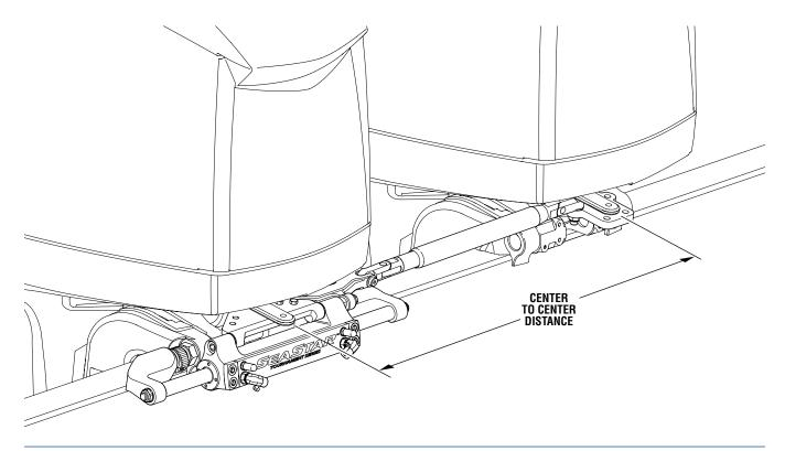
Figure 3-12. Twin Engine – Single Cylinder (Starboard) Configuration.
