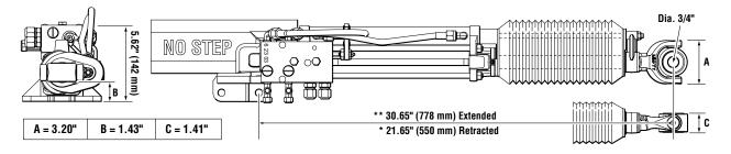
Figure 8-2. \* Add 2" (50 mm) to this dimension for HC5803-2. \*\* Add 4" (101 mm) to this dimension for HC5803-2.
