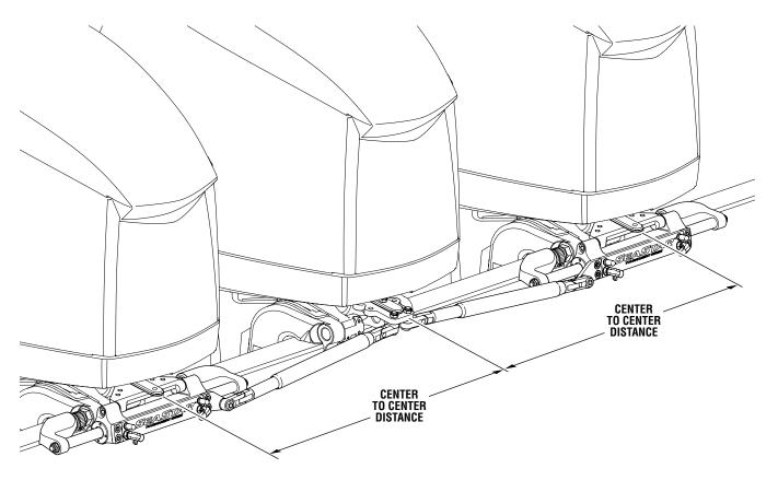
Figure 3-14. Triple Engine – Dual Cylinder Configuration.
