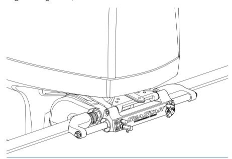
Figure 3-11. Single Engine – Single Cylinder Configuration.
