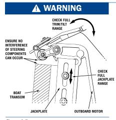
Operational interference of the steering cylinder/cylinder fittings and jackplates/transom/splashwell can occur under certain conditions. Check installation thoroughly throughout the full range of Motor Tilt, Jackplate Height and Trim before making final installation.
