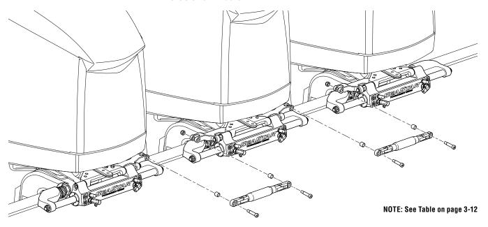
Figure 3-15. Triple Engine – Triple Cylinder Configuration.
