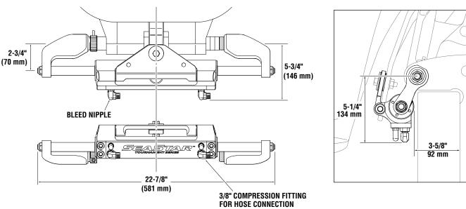
Figure 3-16. Tournament Cylinder Dimensions.
