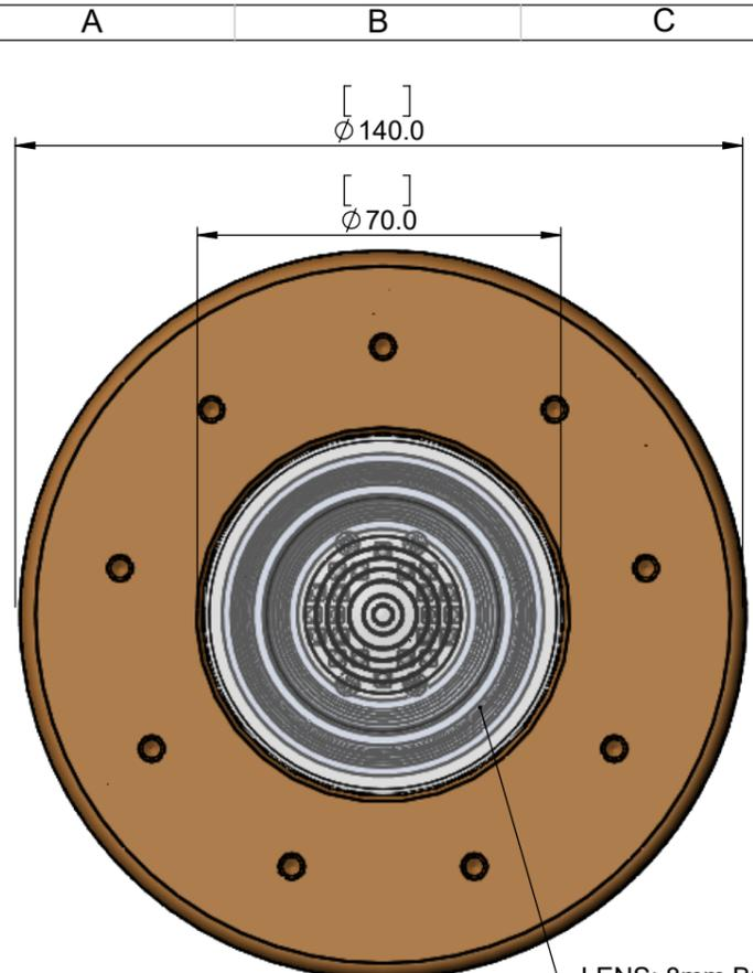
LENS: 8mm BOROSILICATE LENS WITH ANTI-STICK COATING
