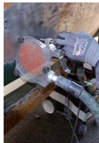
Removing paint with adjustable guide and dust cover
