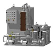
CleanSewage-BIO is a compact, type approved marine Sewage Treatment Plant (STP) for cargo vessels. With an incorporated Moving Bed Bio Reactor (MBBR), the CS-BIO requires minimal processvolume, still meeting the IMO MEPC.227(64) discharge criteria. The accessibility from one side allows ship designers to plan space in the engine room on a whole new level.
