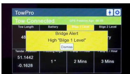
TowPro is described as 'eyes in the boat', and uses innovative data monitoring technology to increase the awareness of crew on watch by providing comprehensive safety data about what is actually happening in the towed vessel. TowPro will automatically trigger audible and visual alerts if any safety indicators exceed pre-set thresholds, providing the crew with immediate early warning of any potential issues.
