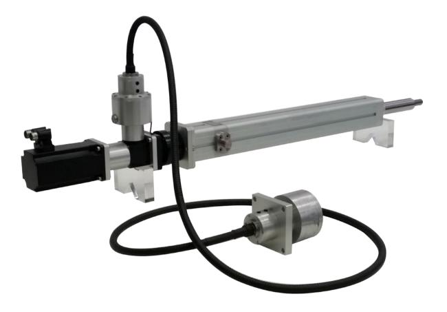
The electrical unit consists of an electric linear actuator, commonly called electro cylinder with a push/pull rod connected to one end of the bar by a support with ball joint. The actuator is fitted to the boat's structure through a cardan joint.
